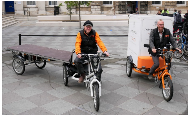
Figure 5-3: Cargo bikes illustrating different configurations (Image courtesy of Tom Bogdanowicz)
